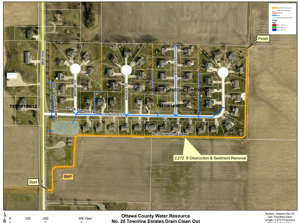
Length: 2,272 ft Cleanout Drain length: 1.02 mi Easement: 20 ft
