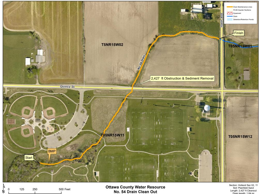
Length: 2,427 ft Cleanout Drain length: 1.64 mi Easement: 0 ft
