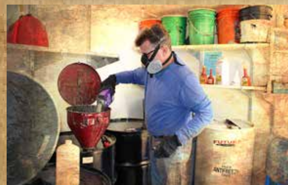
Pour off flammable materials from small containers into 55-gallon drums.
