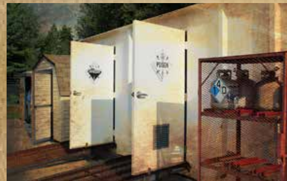
Separate corrosives, poisons and flammables; ensuring they’re in substance appropriate containers, properly sealed and labeled.
