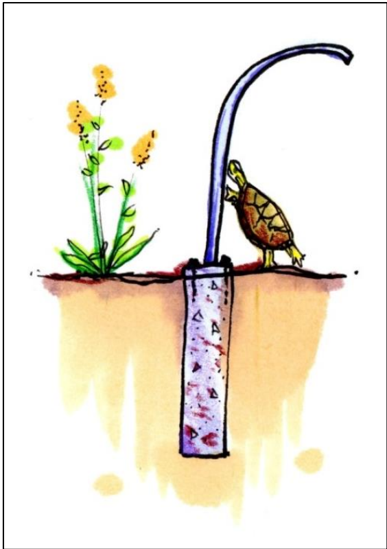
Figure 5. Wildlife barriers which are anchored into the ground prevent amphibians and reptiles from burrowing under or crawling over into roadways or other hazardous areas. Graphic used with permission (Mifsud, D. 2014).
