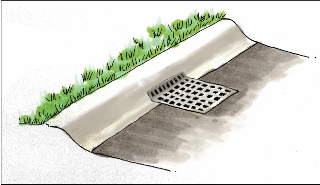
Figure 6. Storm drain grates with smaller openings and grating along the curb prevent amphibians and reptiles from falling through. Graphic used with permission (Mifsud, D. 2014).
