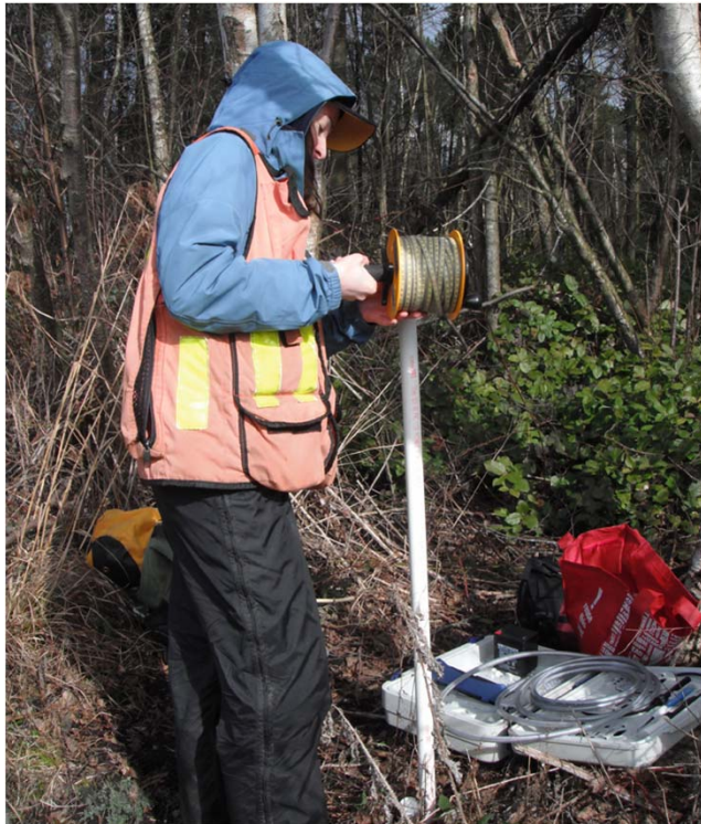
Static Water Level and Chloride Trend Monitoring
